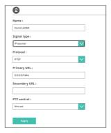
Step 2: Set up the connection of the Microphone system with the DS-9CU in [Speaker Tracking \ Control settings] page. Input the IP address of the Microphone system to add into the list. Please make sure your microphone system is in the AREC official compatible list.
