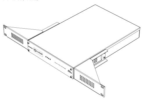
When installing the BLU-DAN into a rack, it is recommended that one empty rack space is left above and below the device. This allows heat to safely dissipate. Furthermore, DO NOT attempt to install two BLU-DAN devices side-by-side into the same 1U rack space – doing so will prevent heat from safely dissipating. See the below diagram for further clarification.
