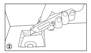
2. Using a utility knife, cut the dampening material and remove it from the inside of the box to expose the conduit knockout. *IMPORTANT! To avoid injury, always wear safety glasses when cutting away dampening materials.*
