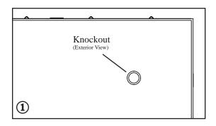
1. On the inside of the backbox (MTC-300BB12) / backcan (MTC-300BB8), locate the general area of the knockout. Note: Because of the dampening material's thickness, you may not be able to feel the wood cut out however, a cut out is located at each knockout point.
