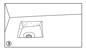
3. Using a hand held punch, strike the knockout and remove the seal.
