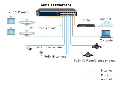
**NOTE:** This switch is designed for indoor use only. If you want to connect to a device located outdoors, the outdoor device must be properly grounded and surge protected, and you must install an Ethernet surge protector inline between the switch and the outdoor device. Failure to do so can damage the switch.
