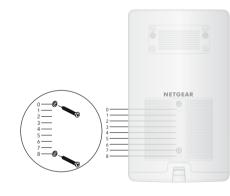
Drill holes into the wall for the two anchors in which you will insert the
