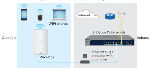
If connected to 2.5 Gbps equipment, the WAX610Y LAN/PoE+ port supports Ethernet speeds up to 2.5 Gbps within your LAN. The preceding figures show a NETGEAR MS510TXUP switch, which supports speeds of 2.5 Gbps and higher, as well as PoE+. If your Internet connection, modem, router, and switch support a speed of 2.5 Gbps, the AP's Internet connection also functions at 2.5 Gbps. Otherwise, the Internet connection functions at 1 Gbps, which is a common speed.
