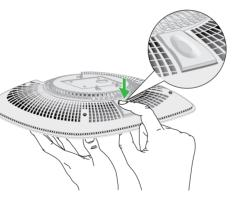
3. Turn the AP counterclockwise until the AP releases from the mounting plate. The mounting plate remains attached to the T-bar or the wall.
