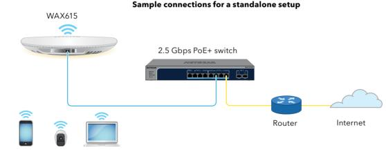
If connected to 2.5 Gbps equipment, the WAX615 LAN PoE+ port supports Ethernet speeds up to 2.5 Gbps within your LAN. The preceding figures show a NETGEAR MS510TXUP switch, which supports speeds of 2.5 Gbps and higher, as well as PoE+. If your Internet connection, modem, router, and switch support a speed of 2.5 Gbps, the AP's Internet connection also functions at 2.5 Gbps. Otherwise, the Internet connection functions at 1 Gbps, which is a common speed.
