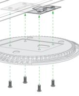
7. Hold the AP upside down and attach it to the mounting plate.
