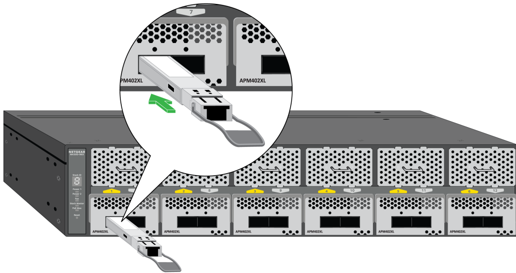
Figure 8. Inserting a QSFP transceiver module
