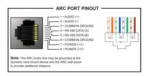
The Symetrix ARC-PSe provides serial control and power distribution over standard CAT5/6 cable for systems with more than 4 ARCs, or when any number of ARCs are located long distances from an Integrator Series, Jupiter or Symetrix DSP unit.
